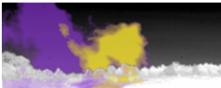
Remote chemical imaging of a simultaneous release of SF 6 and NH 3 at 1.5km using the FIRST imaging spectrometer [22]
